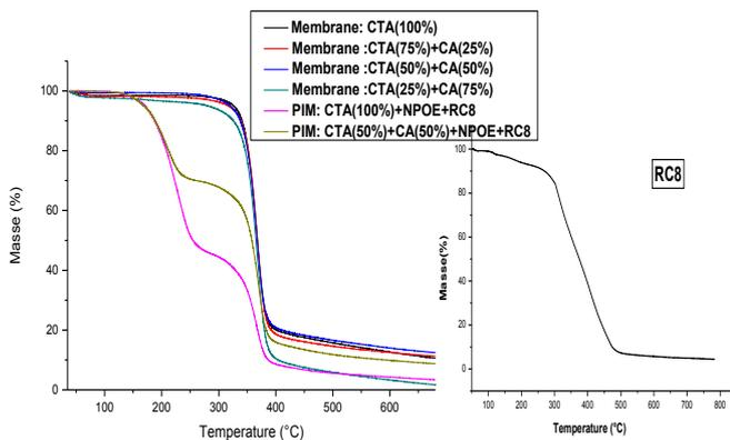
Figure 5. Thermograms of the Membranes, PIMs, and RC8.
