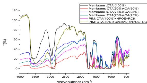
Figure 3. Spectrum of different membranes and PIMs.
