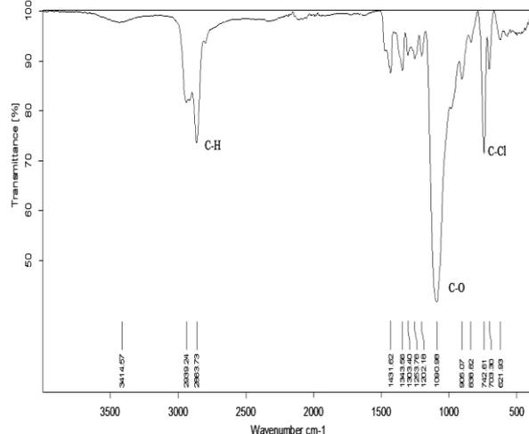
Figure 3. IR spectrum of Poly (ECH-co-THF).
