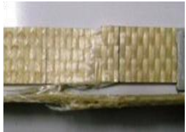
Figure 6. Breaking mode by tensile test of laminate
